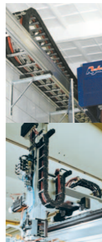
A portal robot equipped with a chain permits reliable, efficient picking, placing and positioning
