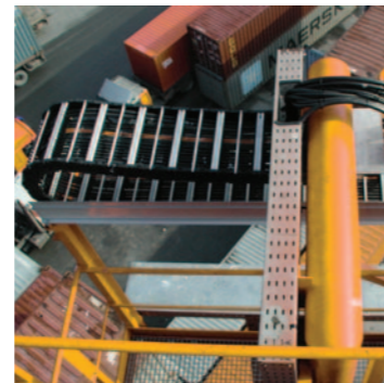
Kabelschlepp energy guiding chain on a port crane
