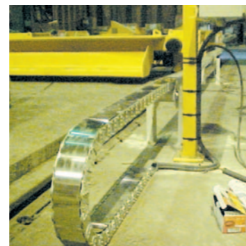
Provides a safe process – Steel chain with covers in a steel mill
